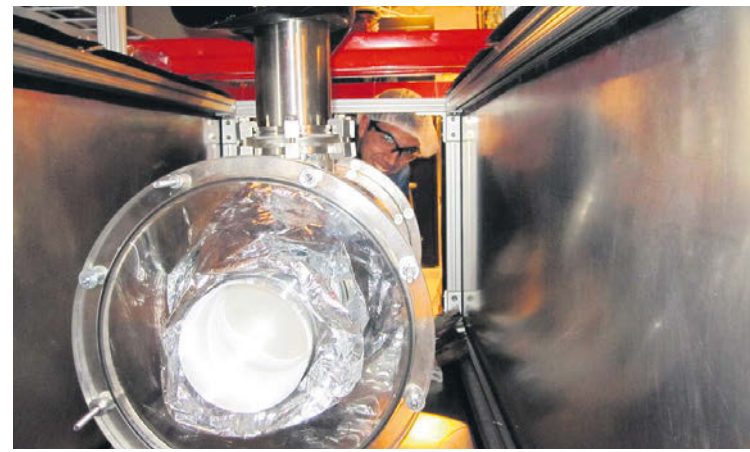
Student Dagoberto Contreras works on the prototype version of the DEAP experiment (left) and the view from above showing the DEAP-3600 experiment under construction (right). This experiment uses 3,600 kilogram of liquid argon to detect dark matter particles. These particles are so non-interactive that this experiment may only see a few per year. SNOLAB
