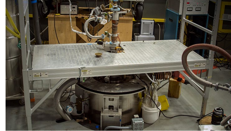
17 Tesla Superconducting Magnet for Optics Credit: National MagLab
